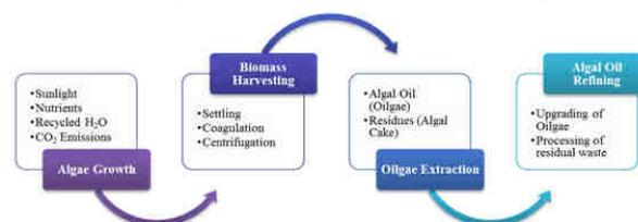
Fig. 1: Algal processing for jet fuel production
